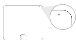
Insert two thumbtacks (not included) into the two holes on the top of the antenna.
