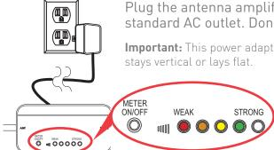
Plug the antenna amplifier's power adapter into a standard AC outlet. Don't connect it to your TV yet.
