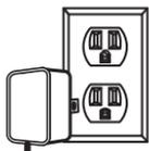
Plug the antenna's power injector power adapter into a standard AC outlet. Don't connect it to your TV yet.
