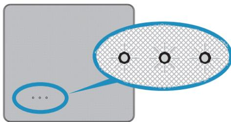
Move your antenna until the signal meter shows at least the second indicator. For best performance, try to get the third indicator.
