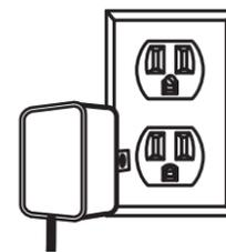
Important: This power adapter should be plugged in so that it stays vertical or lays flat.
