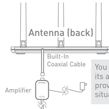
**IMPORTANT:** Don't plug the amplifier's power cord into a power outlet yet.
